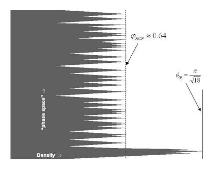
Figure 1: Sketch to illustrate that at the volume fraction of random close packing  $(\phi_{RCP} \approx 0.64)$ , the overwhelming majority of allowed inherent structures disappear. The number of allowed crystalline structures (including structures with defects) is much smaller, and an even smaller number persists all the way up to the density of regular close packing  $(\phi_{cp})$ .
