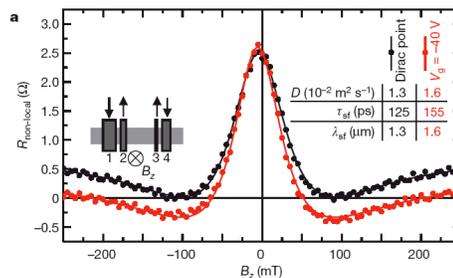
Figure 4a of paper: Electron spin precession induced by out-of-plane B field.
