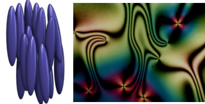
Fig 1: Left – Microscopic picture of nematogens, head-tail symmetric rod like objects that align when densely packed (image courtesy wikipedia). Right – Macroscopic view of a nematic liquid crystal film under cross polarizers showing defect pairs (image courtesy NSF Science360)
