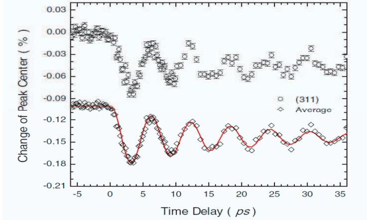
FIG. 1: The ringing of the diffraction pattern due to a standing acoustic wave
