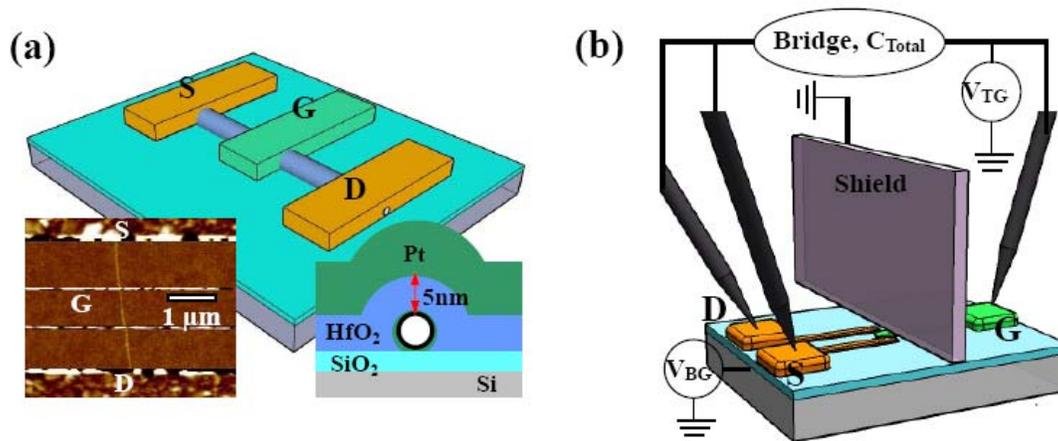
Quantum capacitors: A 5nm HfO<sub>2</sub> dielectric separates a single wall carbon nanotube from a metallic gate. The setup includes careful shielding of the electric field to reduce stray capacitances. (adopted from Yuerui et al.)
