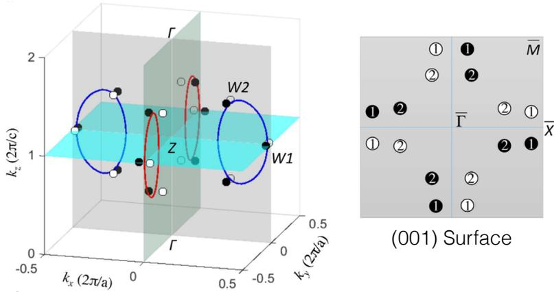
Figure 1: Calculated 3D band structure of TaAs (from [1]) showing the 12 pairs of Weyl nodes. On right, the (001) surface Brillouin zone, with projections of Weyl nodes - some Weyl nodes line up to give a net chirality of  $\pm 2$ . These charges denote the number of Fermi arcs that should emanate from these points.
