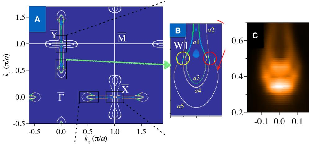
Figure 2: (A). Calculated (001) surface band structure of TaAs. (B). detailed view of part of the calculated band structure. The segment  $a5$  is clearly a Fermi arc. (C). Fermi surface determined from ARPES data in the same part of the Brillouin Zone, showing surface states at the Fermi energy, which can be compared with panel B. (Adapted from Reference 3)
